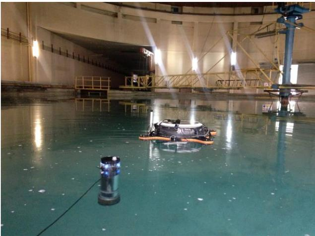
**Fig 1.** aPad surface platform moving to collect and dock aMussel robot.
