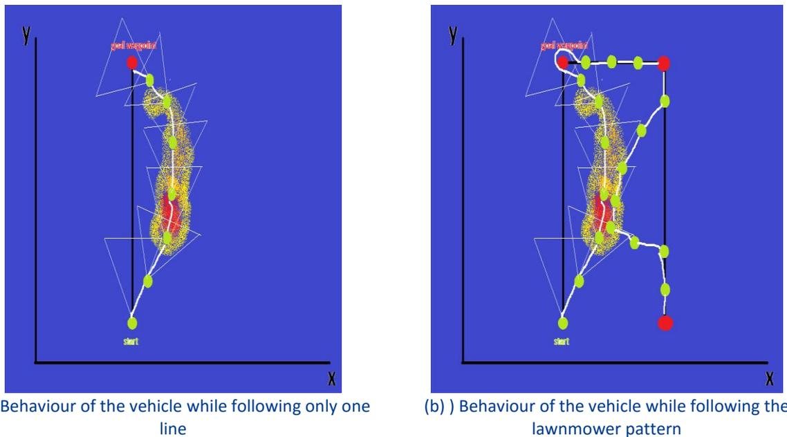
**Fig 1.** Graphical representation of the behaviour of the vehicle. Red points represent the waypoints of the given lawnmower pattern. Green points represent the position of the vehicle in some discrete time moments. The ridge (yellow and red beside the left lawnmower leg) represents some measure of informational gain which the vehicle “collects”.
